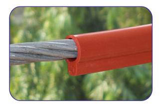
Gala Silicon Interlocking Overhead Line Covers are made from high quality non-tracking silicon rubber that are designed for field installation over bare conductors. These covers provide a layer of electrical insulation for Phase-to-Phase and Phase-to-Ground protection from bird and animals. The GSIOC provides electrical insulation, UV resistance and tracking resistance.
